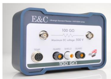
Fig. 3 Developed high-resistance standard resistor, HVR10000 series made by Japan Finechem corporation.
