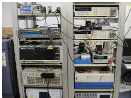
Fig. 5 Photograph of the electrochemical impedance measurement system developed using the Frequency Response Analyzer and the Potentio-Galvano Stat.
