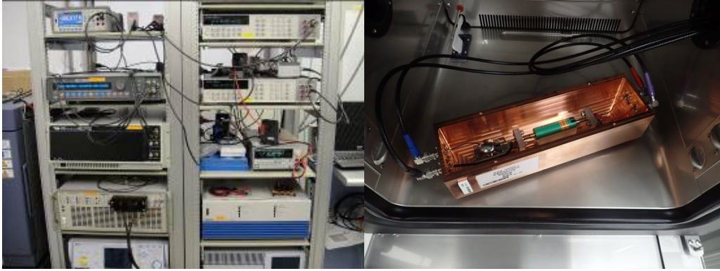
Fig. 4 Electrochemical impedance measurement system and fixture for measuring 18650-type batteries.
