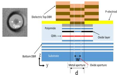
Fig. 2 Metal aperture transverse coupled cavity VCSEL.
