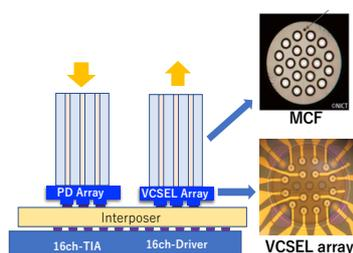
Fig. 1 CPO transceiver based on VCSEL array and MCF.
