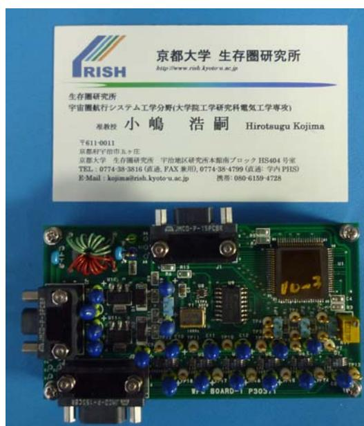
Business card size waveform receiver. The receiver has the capability to observe 6-components of waveforms up to 100kHz, simultaneously.
