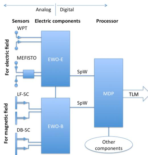
Fig. 2: Overview of EWO block diagram
