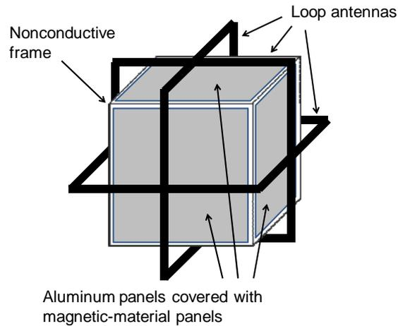
Fig. 3: Configuration of loop antenna system in MSEE node
