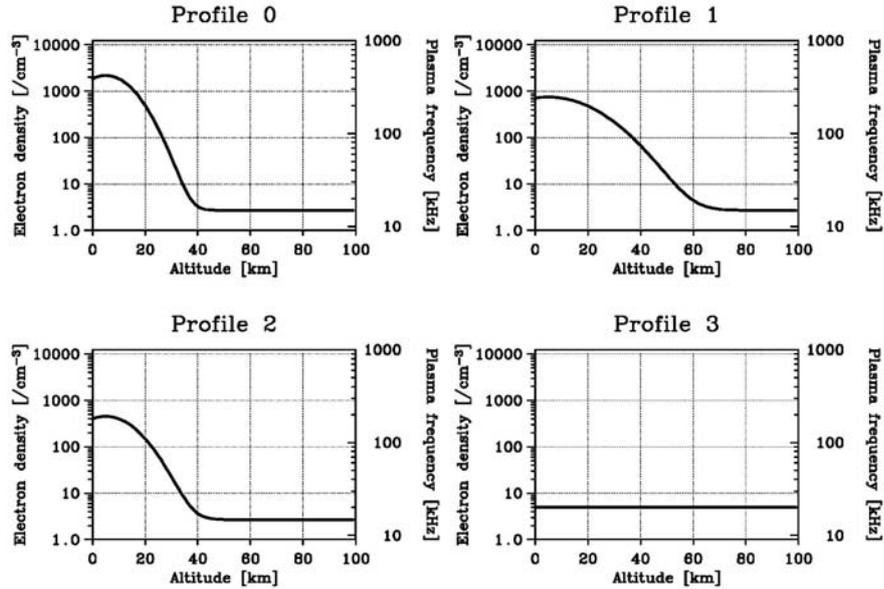
Fig. 1: Electron density model profiles according to Luna 19 and 22 observations (Profile 0, 1 and 2), and a model profile with no ionosphere (Profile 4). [Goto et al., 2011]
