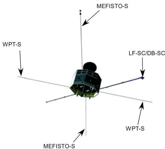
Fig. 1: The sensors aboard MMO for electromagnetic field measurement
