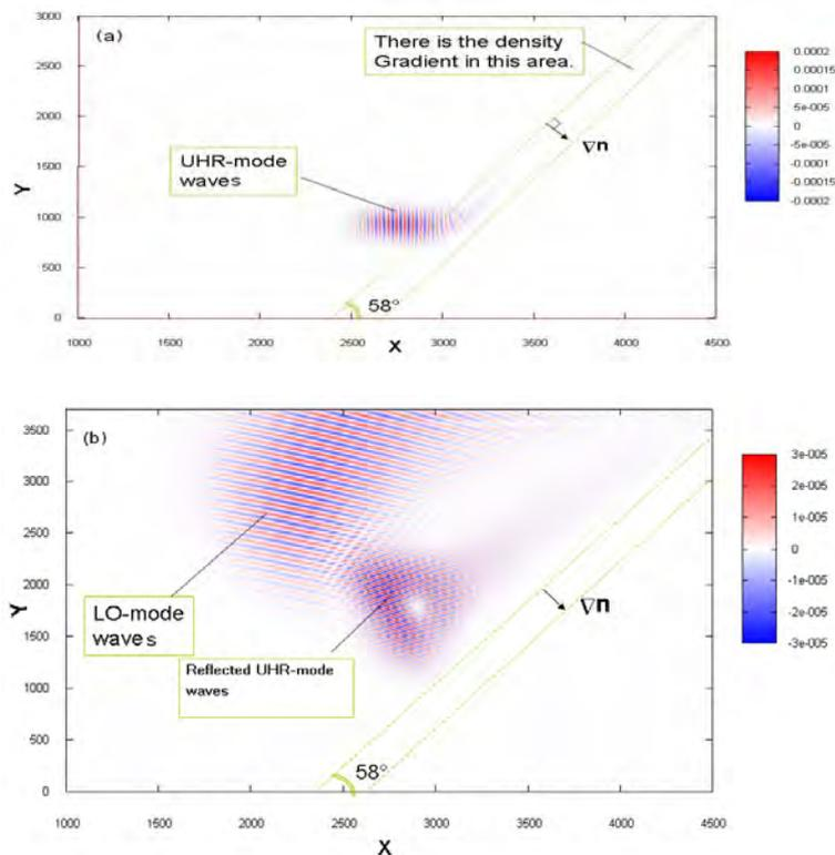
Figure 6. Spatial distributions of the Ex component of the electric field in the simulation system
