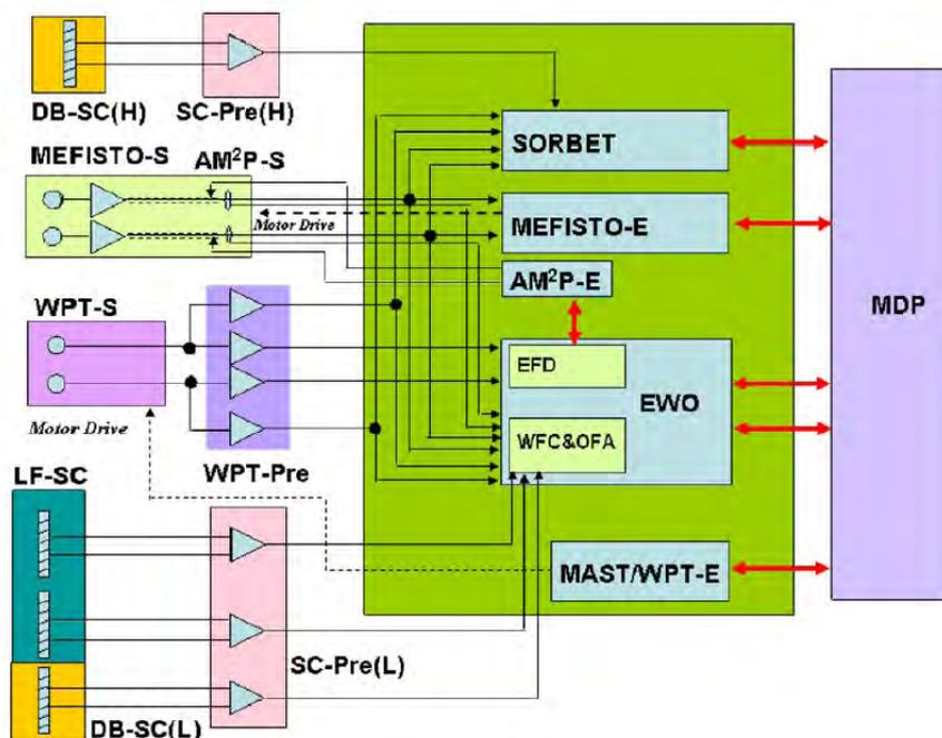
Figure 8. Block diagram of the PWI system onboard the BepiColombo/MMO
