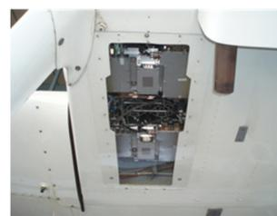
Figure 2. Onboard active phased array antenna.
